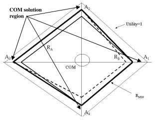
Figure 2. Computation of Center of Mass Region Assume  $R_i(x)$  is dependability requirement for attribute
