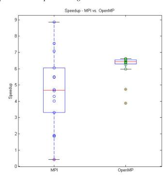
Figure 6: Degree of speedup achieved for MPI and OpenMP development assignments.
