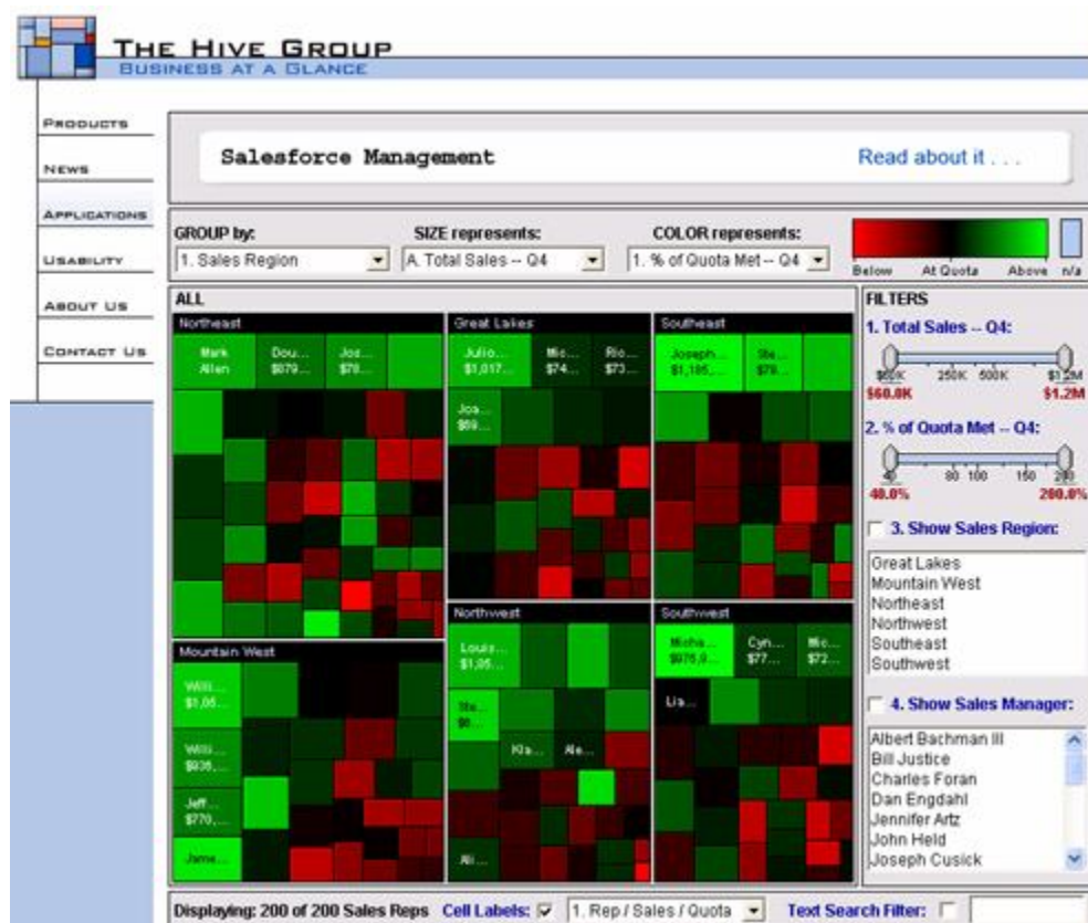
Figure 3: This treemap manages 200 sales representatives, grouped by sales region. Size represents total sales for Q4 and color shows percent of quota met.
