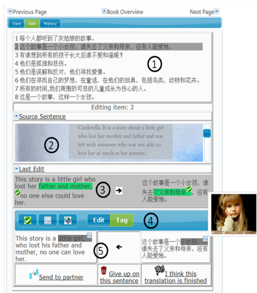
Figure 4. Interface showing an ongoing English-to-Chinese translation. When the user selects a sentence from the list (1), its original source is shown (2) with last edit from the partner (3). The user then edits the sentence with the editor (4). The editor also shows the back translation (5).
