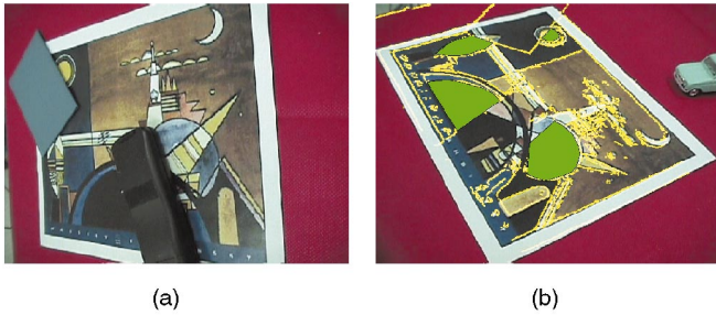
Fig. 11. (a) A new picture of the Kandinsky with occlusion. (b) The pose that is determined using the four shaded regions (the sun, the tree top, and both domes), which are all partially occluded.
