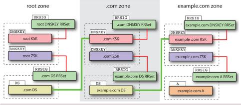
**Figure 1:** Overview of DNSSEC records necessary to validate example.com's "A" record. Each RRSIG is the signature of a record set (dashed lines) verified with a DNSKEY (thinner solid lines). Each DS record is the hash of a child zone's KSK, or key-signing key (thicker solid lines).
