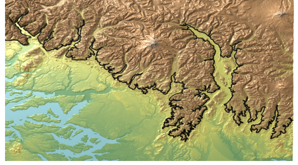
Figure 4: Puget Sound contour line: This image shows a contour line (in black) extracted from an unstructured terrain model of the Puget Sound. The terrain is simplified down to 143M triangles. We extracted the largest component (223K edges) of the level set at 500 meters of elevation. Our cache-oblivious layouts improve the performance of the isocontour extraction algorithm by more than an order of magnitude.
