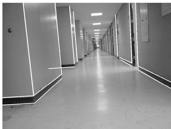
Figure 3: Determining the pose of a CAD model from a real image. Straight lines are automatically detected in the image (top). The initial guess for the pose of the hallway model differed from the true pose by about 14^\circ about each coordinate axis (middle). The projection of the model after finding its pose with our algorithm (bottom).
