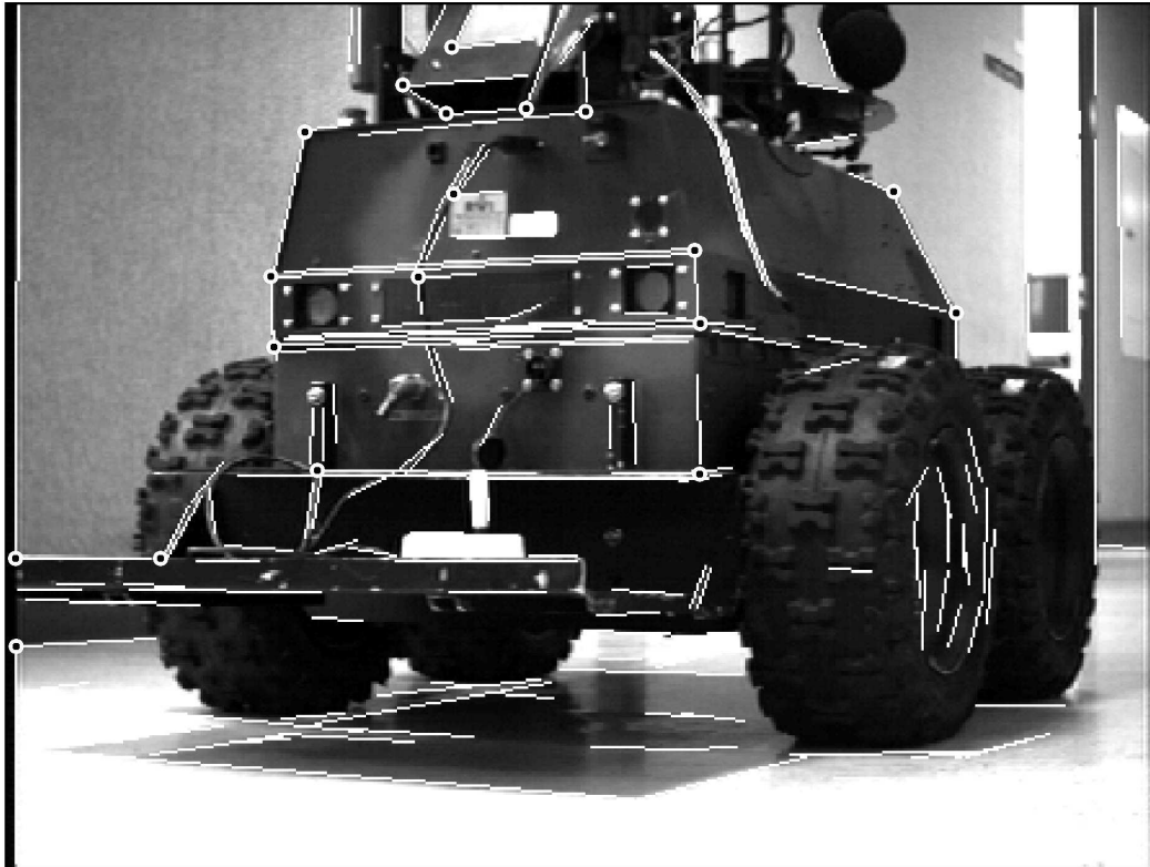
Figure 14: An image of the large robot as seen from the small robot's point of view. Long straight lines detected in the image are shown in white, and their intersections, which ideally should correspond to vertices in the 3D model, are shown in black.
