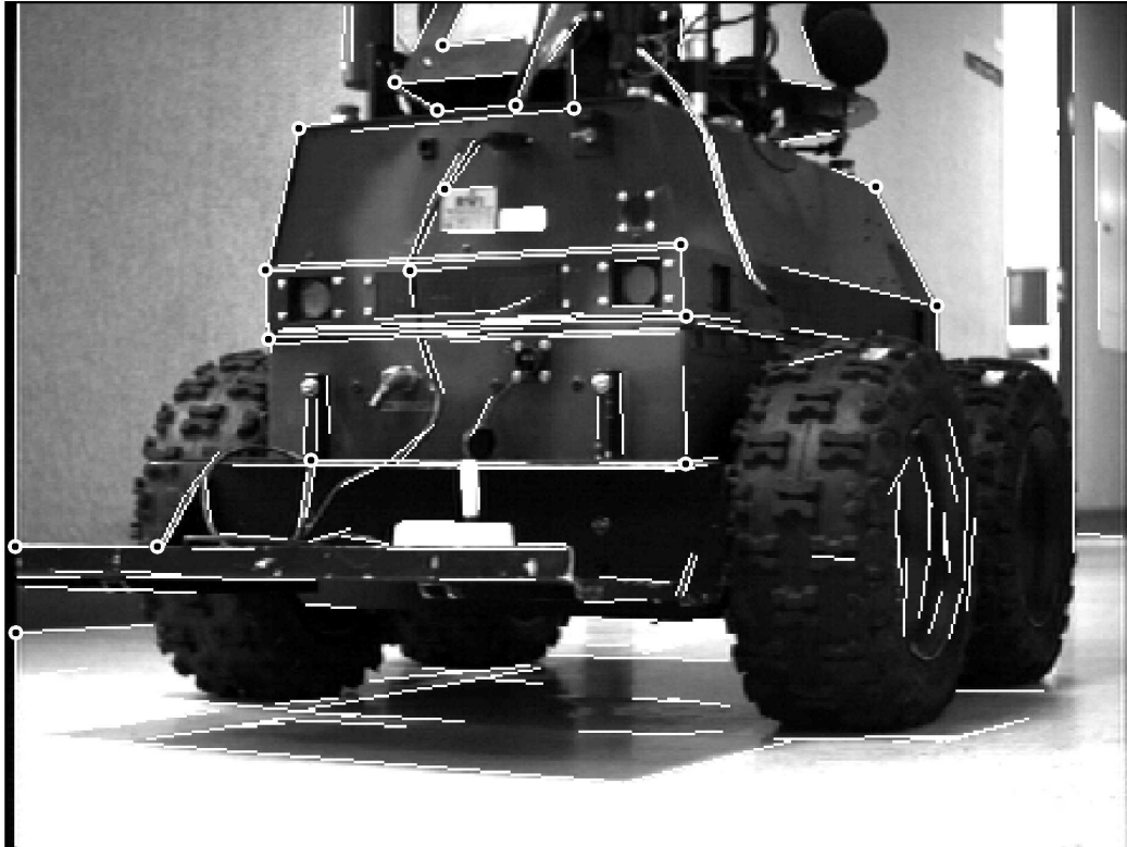
Figure 16: An image of the large robot as seen from the small robot's point of view. Long straight lines detected in the image are shown in white, and their intersections, which ideally should correspond to vertices in the 3D object, are shown in black.
