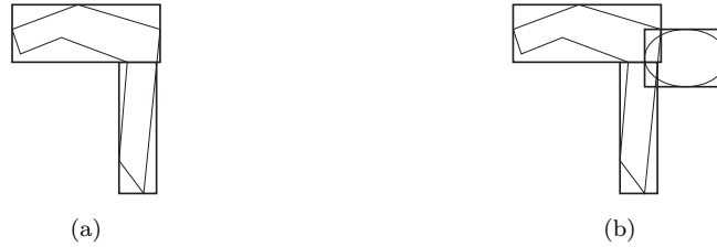
Fig. 21. (a) In order to reduce dead space, an object can be approximated by two disjoint rectangles. (b) However, both rectangles might intersect a second object, thereby producing duplicate results.
