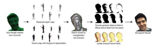
Figure 2. The workflow of the Montage4D rendering pipeline.
