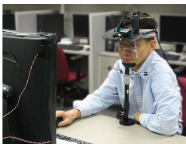
Fig. 1. Our experimental setup for the user study with the ISCAN ETL-500 eye-tracker.
