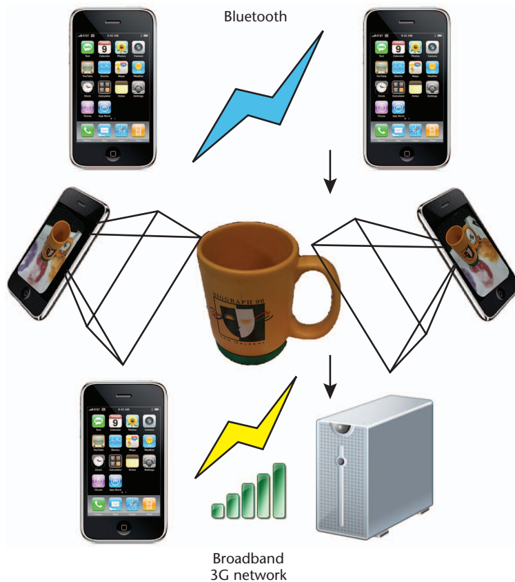
Figure 3. During the acquisition phase, Social Snapshot connects the iPhones in a peer-to-peer network using Bluetooth. This network enables the synchronized acquisition of photographs among the participating devices. The system then uploads the resultant data to the reconstruction server using the broadband 3G network.
