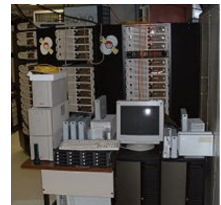
Beowulf computer cluster (Borg, 52-node cluster used by McGill University Image/Info from Wikipedia )
