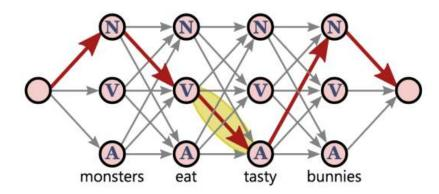
We can use Viterbi algorithm as before as long as the loss function decomposes over the input consistently with features!
