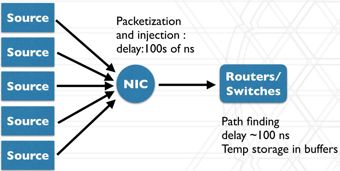
Message origin points : destination, frequency, size, etc. determined by application I micro sec - 10s of sec
