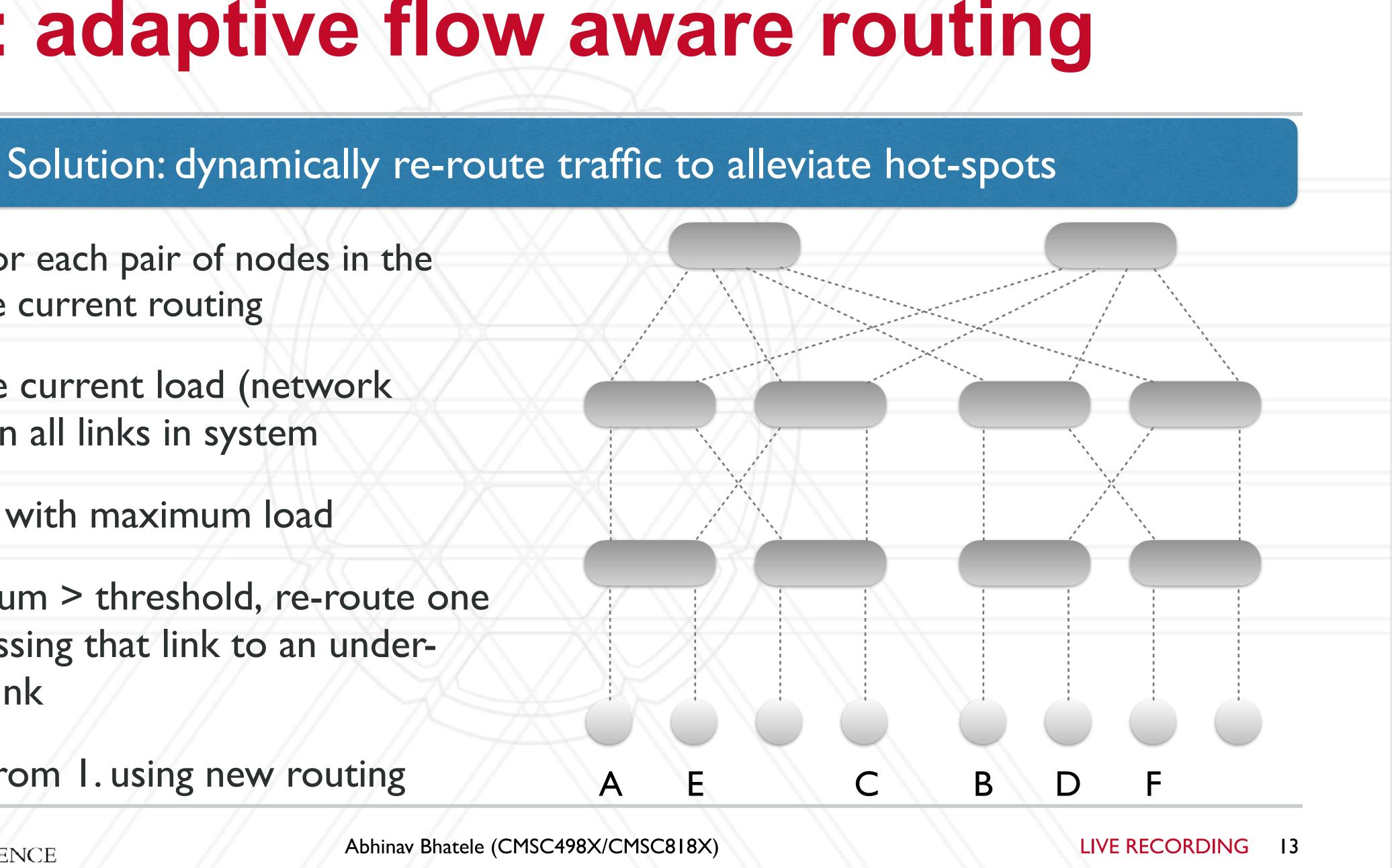
Given: traffic for each pair of nodes in the system and the current routing
