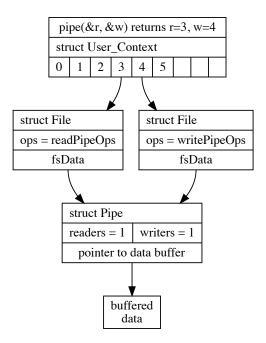
Figure 1: Illustration of the file descriptor table (top), where entries point to struct File objects. There are two struct File objects for the pipe. The pipe object must track whether there are any readers or writers and keep buffered data.
