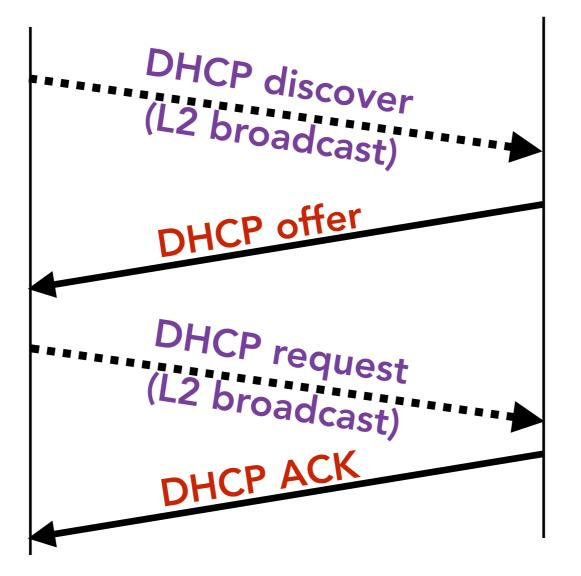
offer includes: IP address, DNS server, gateway router, and duration of this offer ("lease" time)
