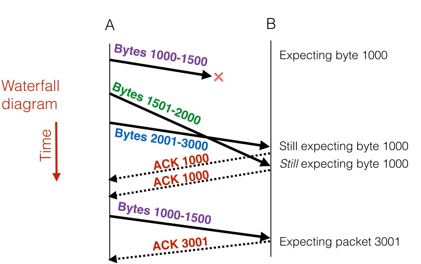
Bytes 1000-1500 Expecting byte 1000 Bytes 1501-2000 Waterfall diagram Bytes 2001-3000 Still expecting byte 1000 Still expecting byte 1000 Buffer these until Bytes 1000-1500 **ACK 3001** Expecting packet 3001
