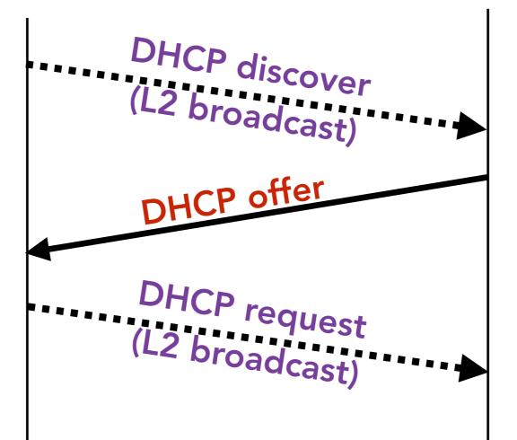
offer includes: IP address, DNS server, gateway router, and duration of this offer ("lease" time)
