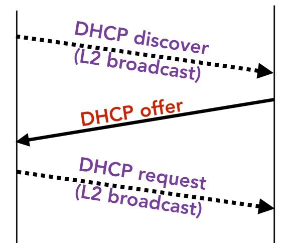
offer includes: IP address, DNS server, gateway router, and duration of this offer ("lease" time)
