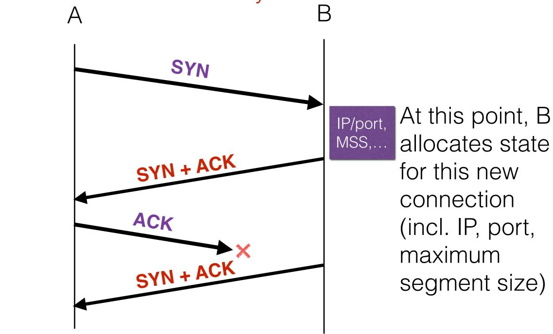
B will hold onto this local state and retransmit SYN+ACK's until it hears back or times out (up to 63 sec).
