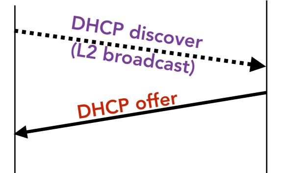
offer includes: IP address, DNS server, gateway router, and duration of this offer ("lease" time)
