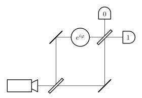
Analyze the experiment depicted above using the mathematical model described in class. (Note that the model from class differs slightly from the model described in the textbook; in particular, you should use the matrix  $\frac{1}{\sqrt{2}}\begin{pmatrix} 1 & 1 \\ 1 & -1 \end{pmatrix}$  to model the beamsplitters.)
