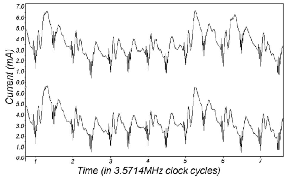
Figure 3: SPA trace showing individual clock cycles.
