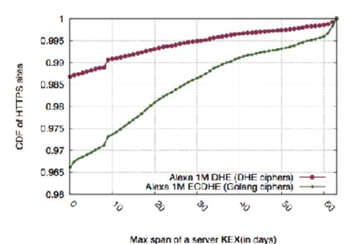
Figure 5: Ephemeral Exchange Value Reuse—We measured how long Alexa Top Million websites served identical
