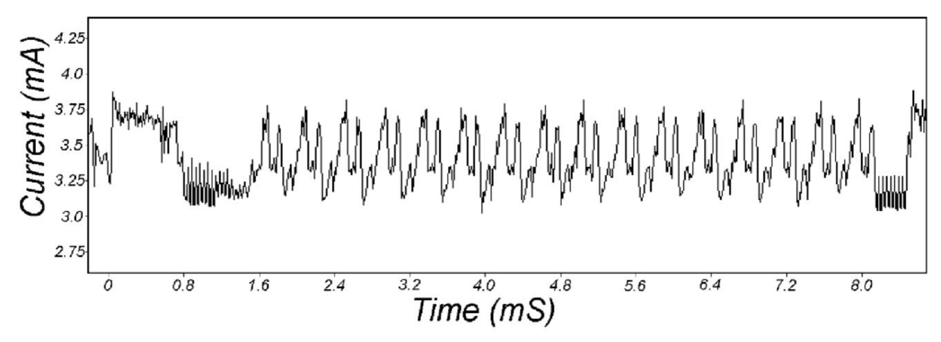
Figure 1: SPA trace showing an entire DES operation.
