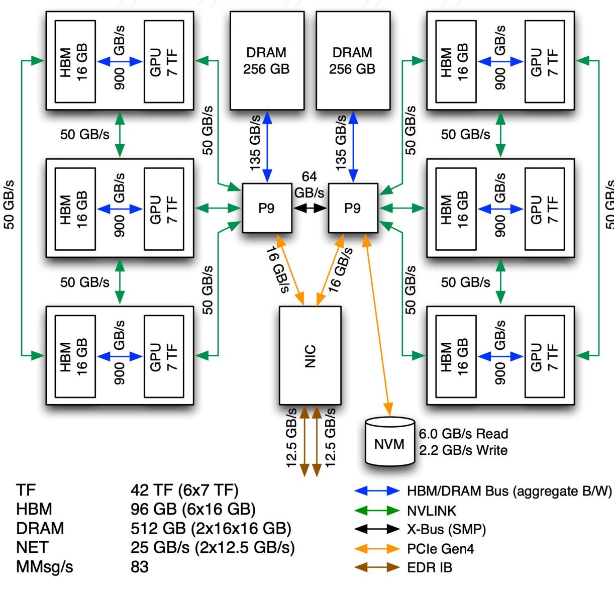
HBM & DRAM speeds are aggregate (Read+Write). All other speeds (X-Bus, NVLink, PCIe, IB) are bi-directional.
