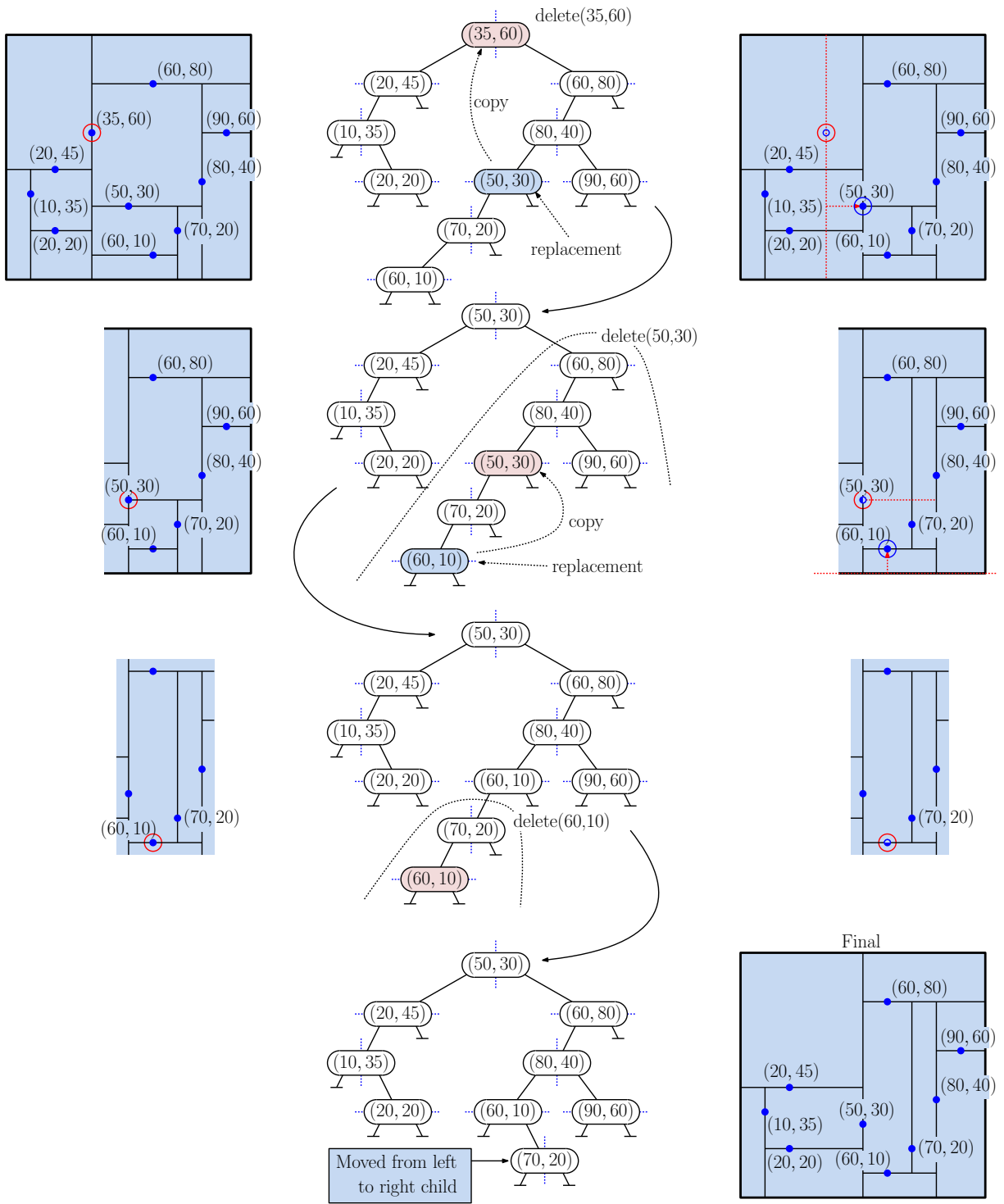
Fig. 64: Deletion from a kd-tree.
