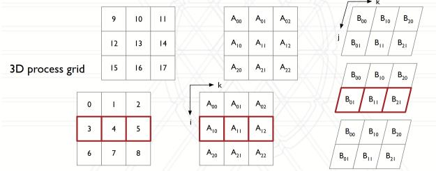
We choose a 2D plane to contain a full copy of the matrix A. In the example, the (i,k) plane contains A, which means we split A into 9 blocks. Each (i,k) slice will contain the same configuration of A. For example process 0 and 9 will have the same sub-block of A, A\_00.
