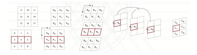
The main differences between Cannon's and Agarwal's is that Cannon's uses less memory since there is only a combined single copy of both A and B but there are more data movements compared. In Agarwal's there are only 2 data movements. The first is a bcast across a plane (but a single process is not sending to all other processes) and the second is an all reduce from multiple processes to a single process.
