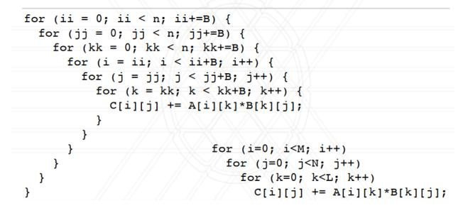
So far we talked about how to compute a more efficient matrix multiplication, but only serially. We now move to parallelizing it. We have to figure out how to efficiently store data, in this case the matrices A and B in a distributed manner, and how to efficiently split up the work to compute the product C and to minimize the communication between the processes.
