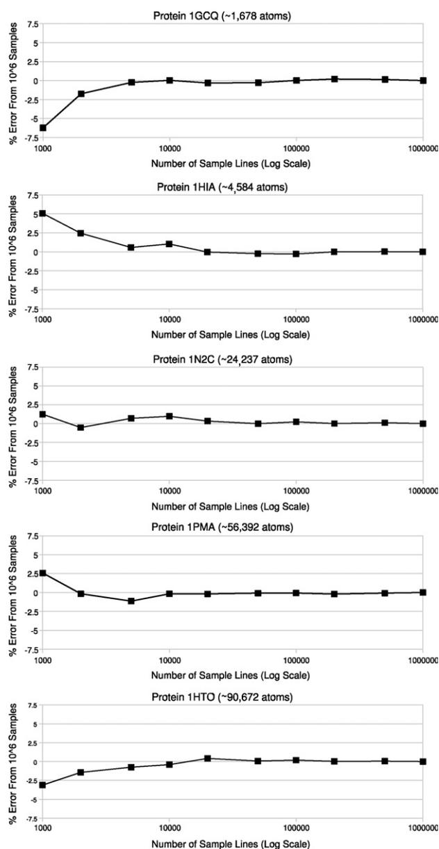
Fig. 1. Surface area approximation errors for several proteins using various numbers of intersected lines. Vertical axis is the percent error from the final value (the area returned with  $10^6$  sample lines). Note that all proteins have converged to near their final area by 20,000 lines.
