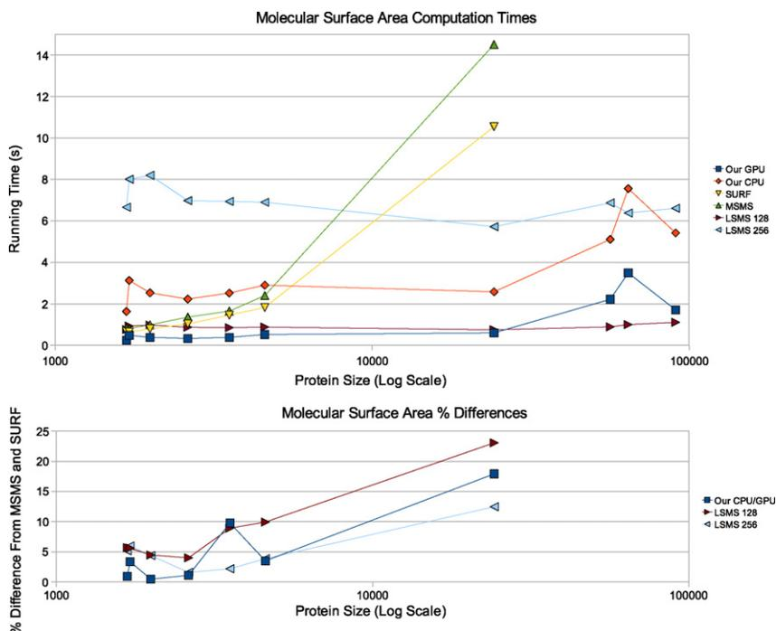
**Fig. 2.** Surface area computation times and percent differences for proteins of different sizes using several different algorithms. Data is from Table 1. Protein size is given in RBFs, which is equal to the number of atoms listed in the PDB file. For MSMS and SURF, data is not available for the larger proteins since these programs were unable to compute the area for proteins of that size. Percent differences are given as absolute magnitudes.
