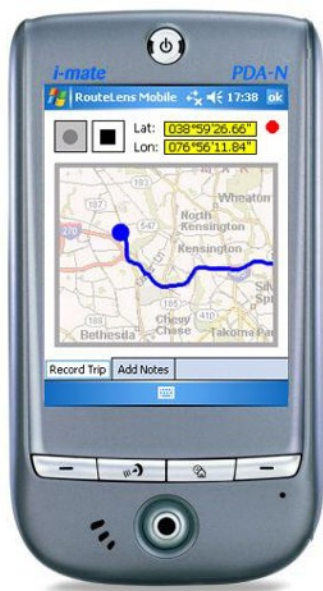
Figure 3: Mobile interface. Simple buttons start and stop recording, labels display position, and map shows route (updating route view only partially implemented)
