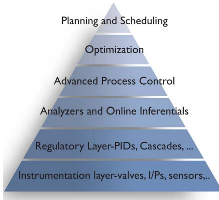
Figure 1 - Plant Process Control Hierarchy
