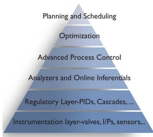
**Figure 3: Plant Process Control Hierarchy**
