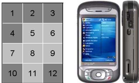
Figure 5: (a) Input regions (dark="hard to reach", light="easy to reach"). (b) The Cingular 8525.
