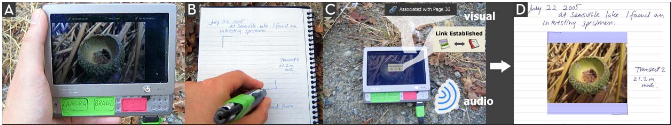
Figure 3. To use hotspot association, a user A) captures or browses to a photo, then B) draws the hotspot gesture into the notebook using the digital pen. C) The smart camera provides real-time visual/audio feedback to confirm the association. D) The ButterflyNet Browser renders the associated photo within the hotspot brackets, inline with the digitized notes.
