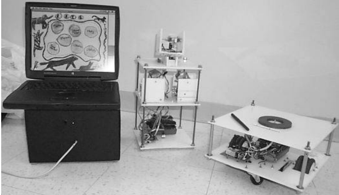
Figure 7: the MyPETS software, the transmitter box, and the skeletal components of PETS 2
