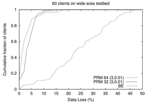
**Figure 8: Cumulative distribution of data losses for a 30 minute experiment on a group with 60 clients (on average) performed on the wide-area testbed. The overlay node failure and join rate was 4.8 per minute each.**
