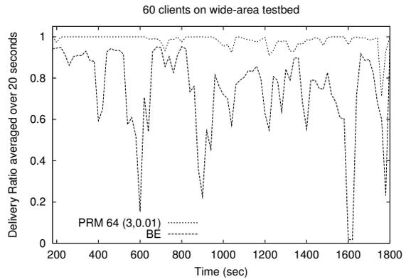
**Figure 7: Data delivery ratio achieved by a group of 60 clients (on average) on the wide-area testbed for a 30 minute experiment. The media stream was started three minutes into the experiment. The data delivery ratio is averaged over each 20 second interval for clarity. The overlay node failure and join rate was 4.8 per minute each.**
