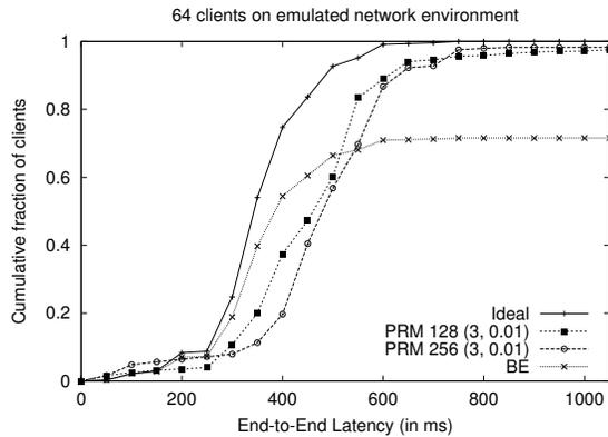
**Figure 6: Distribution of latency experienced at the clients for a group of 64 nodes (on average) with overlay node failure rate and join rate of 4.8 per minute. Ideal marks the latency distribution for a hypothetical scenario when the overlay paths to the clients are instantaneously repaired following a failure or a join, i.e. there are no data losses on the overlay path.**
