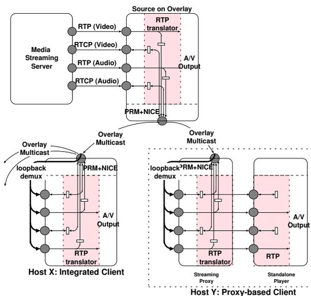
Figure 2: RTP and RTCP paths in SRMS.
