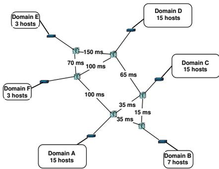
**Figure 3: The network topology used in the emulated network environment. Each backbone link is marked with the average latency. The losses on the links connecting the access gateways and the backbone were chosen randomly between 1% and 2%. Within each domain the latencies between pairs of hosts were randomly assigned between 5 and 10 ms, and the corresponding losses were 0.2% to 0.5%.**
