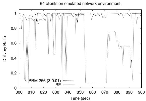
**Figure 4: Data delivery ratio achieved for a group of 64 clients as they join and leave the multicast group. Overlay node failure and join rate was 4.8 per minute. Between time 850 and 860 seconds four intermediate overlay nodes on the data delivery tree left the multicast group.**
