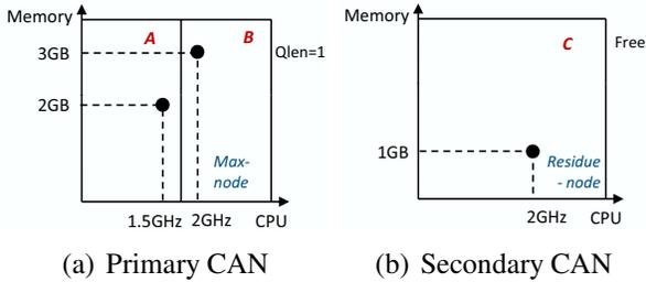
**Figure 2. Dual-CAN: Node *B* creates a Residue-node *C* on the Secondary CAN**
