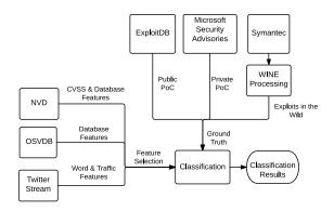
Figure 1: Overview of the system architecture.
