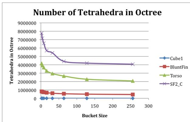
Figure 5: Number of tetrahedra in bucket PR octree for each mesh
