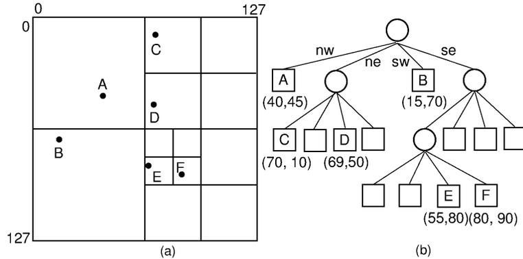
Figure 1: PR quadtree with six vertices
