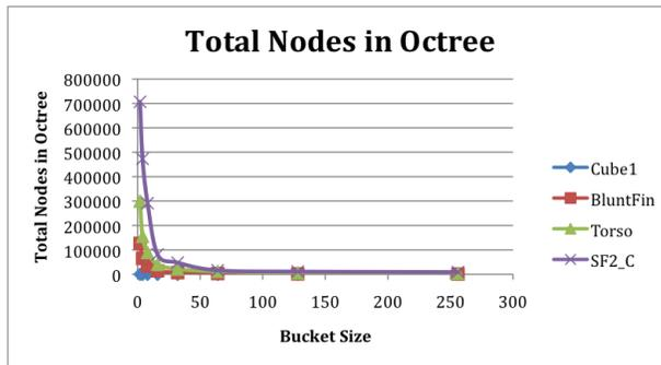
Figure 8: Amount of total nodes in the bucket PR octree for each mesh
