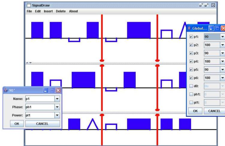
Figure 1: Screen capture of SignalDraw. The main screen, pulse property, and global properties windows are shown.
