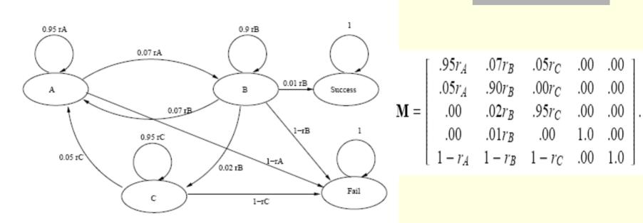
A module reliability diagram, where  $r_A$ ,  $r_B$  and  $r_c$  are the reliabilities of the modules A,B and C.
