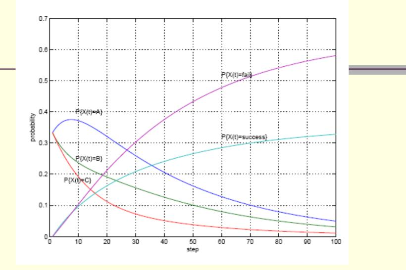
Figure shows how the probabilities of each states change over time and how the reliability of the program (P{X(t) = success}) is accumulated with the module reliabilities  $r_A$ ,  $r_B$  and  $r_C$  and initial pmf x(0) = [1/3,1/3,1/3,0,0]
