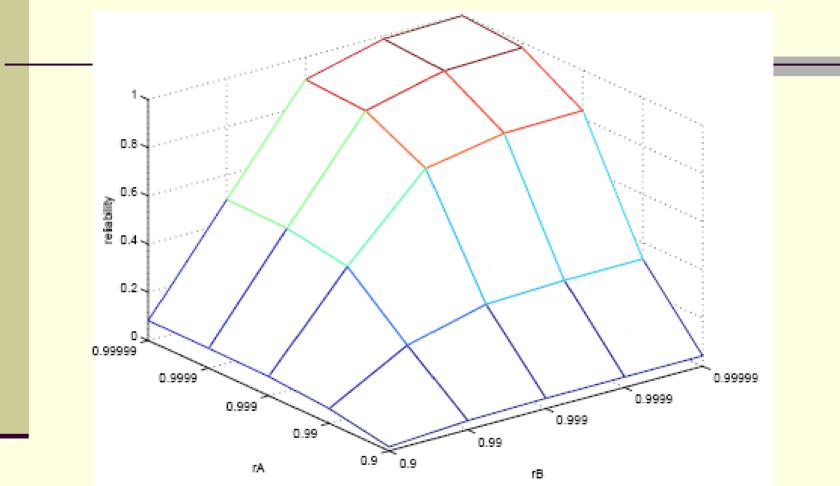
Reliability of a program as a function of module Reliabilities  $r_A$  and  $r_B$  with  $r_c = 1 - 10^{-5}$ Transition probabilities significantly affect the overall reliability of the program.
