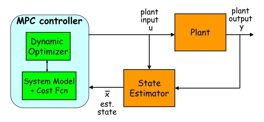
*Goal:* compute an optimal input by minimizing given cost function over a certain prediction horizon using model of the system
