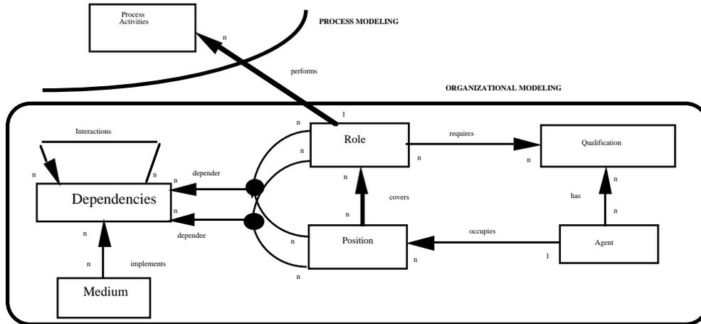
Figure 4: Modified ER model for AD graphs
