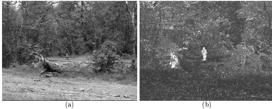
Fig. 4. Background Subtraction. (a) original image. (b) Estimated probability image.
