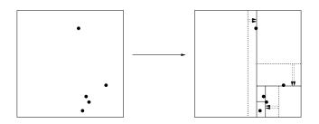
Figure 2: Example of the sliding-midpoint rule.
