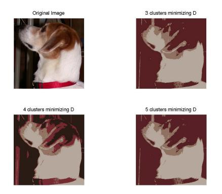
Figure 11.3. The images resulting from minimizing D.
