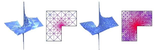
Stokes flow over an L-shaped domain: Pressures and meshes for error tolerance of 5% and unstable finite element pairs (resp. DOFs):  $\mathcal{P}^2 - \mathcal{P}_d^1$  (1940),  $\mathcal{P}^1 - \mathcal{P}^1$  (4971). The oscillations do not persist under further selective refinement (nonlinear stabilization effect of adaptivity). Error estimation and adaptivity will be fully discussed in this course.
