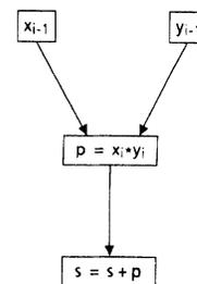
Fig. 1. Systolic array for the inner product.
