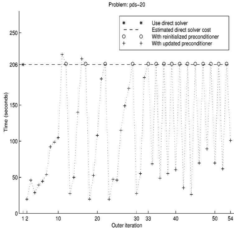
Figure 3. Timing performance for the adaptive algorithm on problem `pds-20`.
