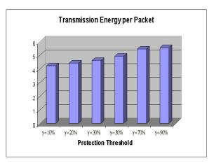
Fig. 9. CMRPC: Avg. Transmission Energy per Received Packet vs.  $\gamma$
