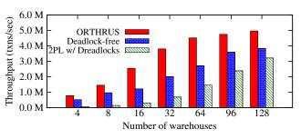
Figure 8: TPC-C NewOrder and Payment throughput, varying number of warehouses. Each system uses 80 CPU cores.
