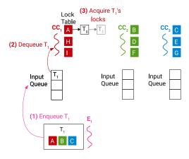
Figure 2: Concurrency control thread acquiring locks on behalf of an execution thread.
