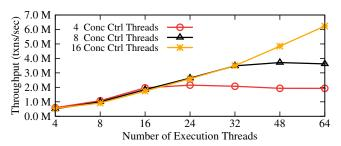
Figure 5: Execution thread scalability in ORTHRUS under various fixed concurrency control thread configurations.
