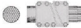
Detail of Main Cable and Cable Band. The wrapping wire is omitted at the right for clarity. Note the closed construction and aluminum fillers.
