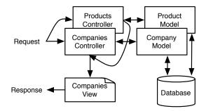
Figure 2. Rails MVC architecture
