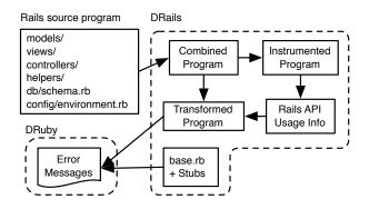
Figure 5. DRails architecture
