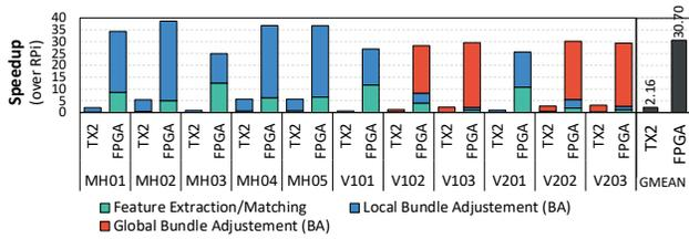
**Figure 17: ORB SLAM speedup over RPi for TX2 and FPGA by category: feature extraction and bundle adjustments.**
