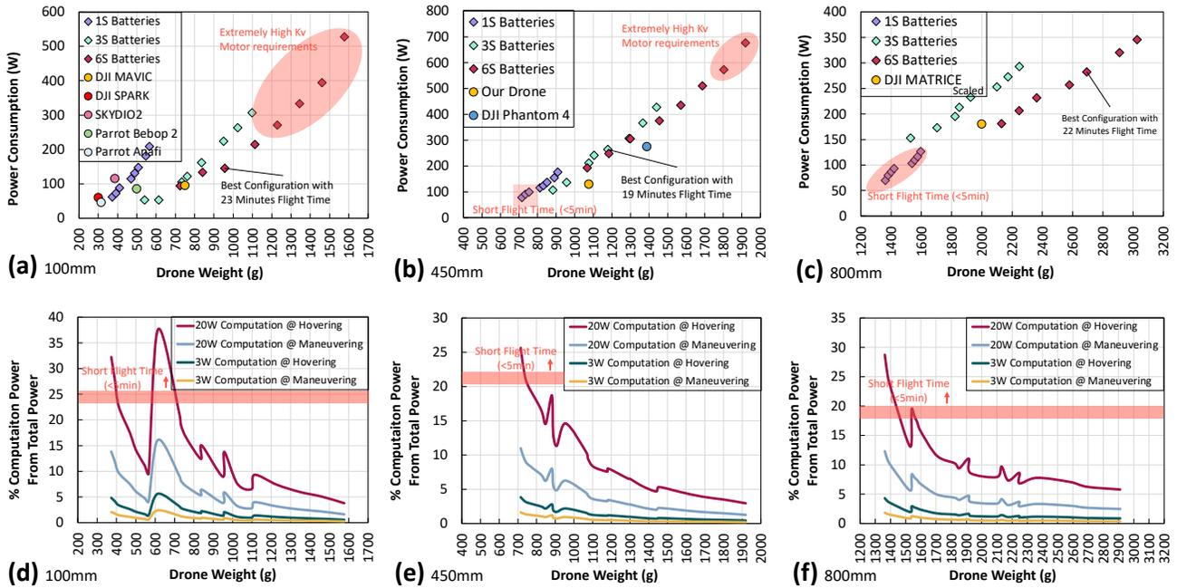
**Figure 10: Top Row (a,b,c):** The total power consumption of drones with various wheelbases extracted by relationships in Equation 3.2 and verified with data from commercial drones shown as additional data points [33, 52–56]. **Bottom Row (d,e,f):** The computation footprint considering 3 W and 20 W chips shown with 3/20W computation @ hovering/maneuvering lines.
