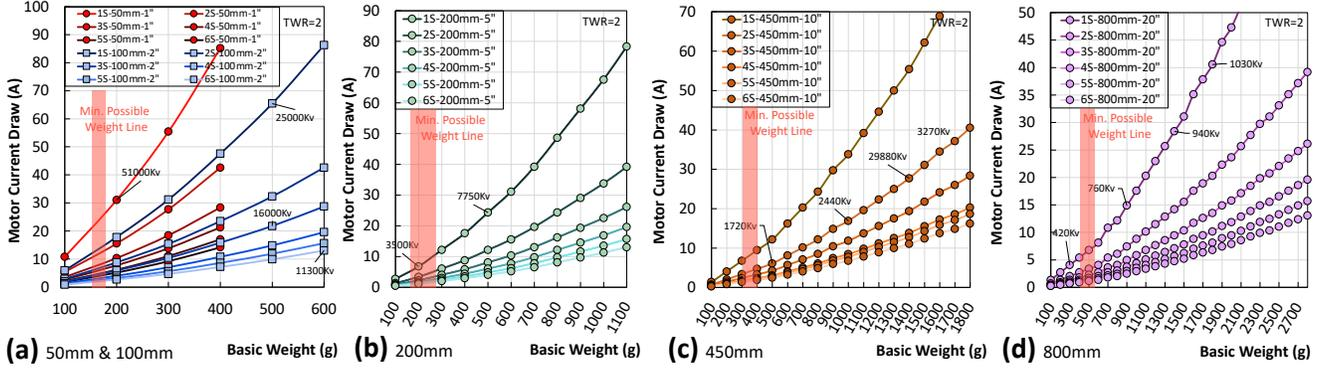
**Figure 9: Relationship between the max per-motor current draw and the basic weight, grouped by supply voltage and wheelbase sizes from 50mm–800mm. TWR is 2 and data is extracted from 150 manufacturers.**
