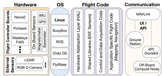
**Figure 5: Hardware-software stack abstraction of a drone.**
