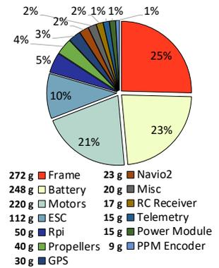
Figure 14: Our drone weight breakdown.
