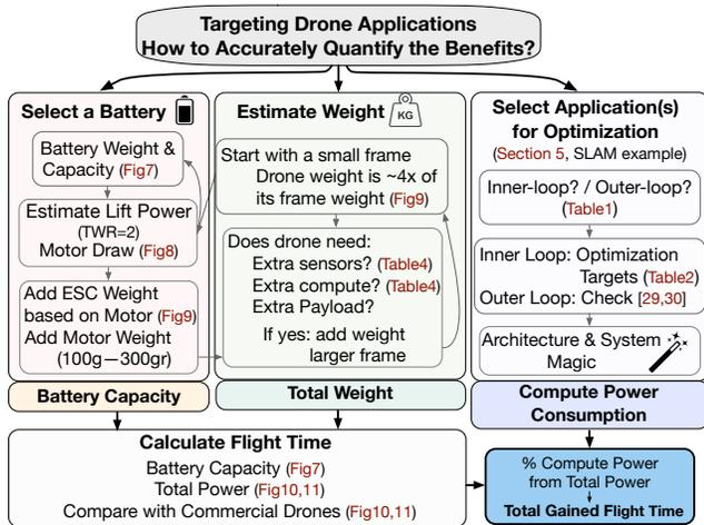
Figure 12: Procedure of quantifying total/compute power consumption in drones.
