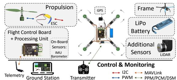
Figure 3: General overview of an autonomous drone.
